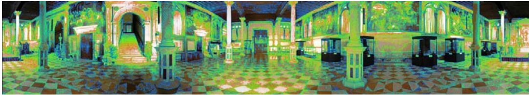
Figure 5 – Video 2 http://dx.doi.org/10.1117/12.2020535.2 Measured luminance of ground level gallery under real lighting condition given a viewing direction, Video 3 http://dx.doi.org/10.1117/12.2020535.3
